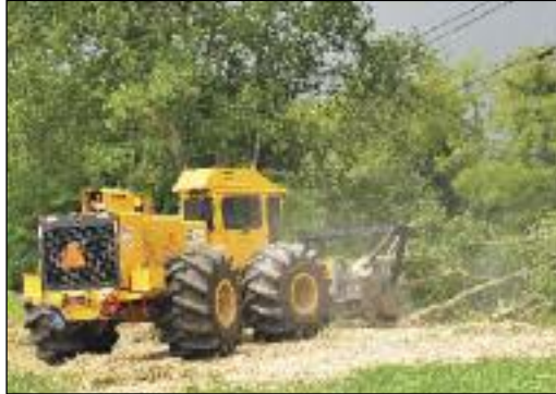
The Kershaw machine quickly clears the electric right of way to remove trees and brush from underneath the power lines.
